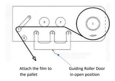
1 – Film Roll 2, 4, 6 = Door Guiding Roller 3 = Brake Roller 5 = stretching Roller
