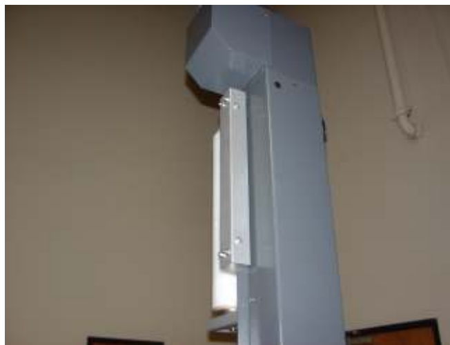
Film carriage at top of mast.
